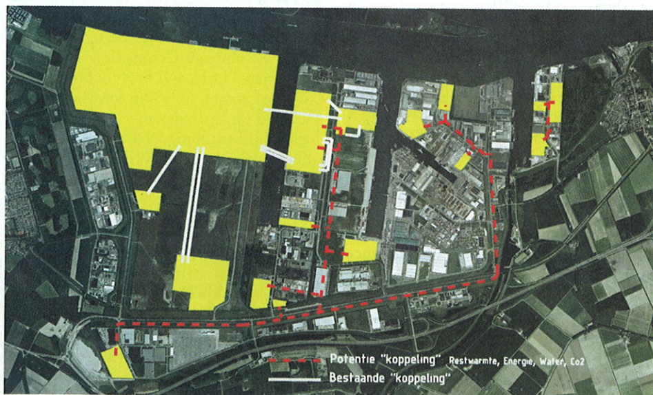
The map provides a picture of the links already established and the links that are possible with regard to the exchange of steam, hot water and CO 2 . Within the next two years, new links will be established.
